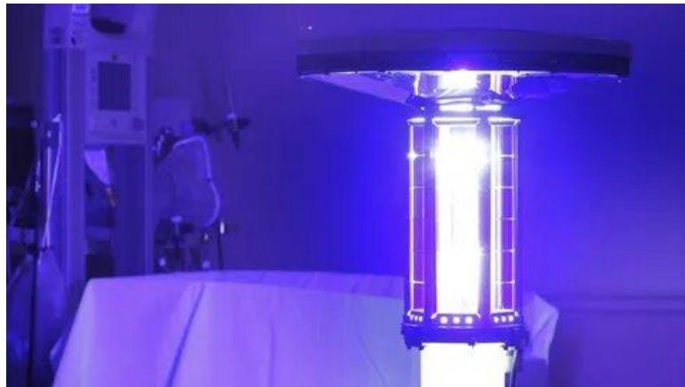
Pic. 1 UV - lamp of open type.
