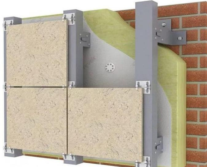
Figure 2. Ventilating facade design
