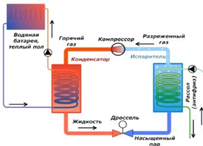
Figure 1. The principle of operation of the heat pump
