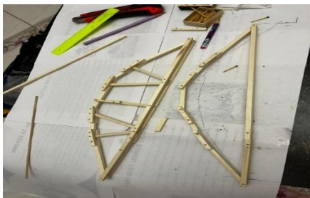
Figure 11. Fabrication of Bridge Arches Figure 12. Bridge Load-Bearing Structure
