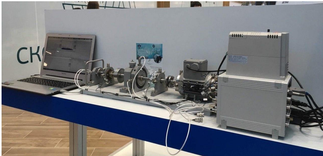
Figure 1. Electromechanical rotor installation with the ability to simulate fault signals of rotating assemblies.
