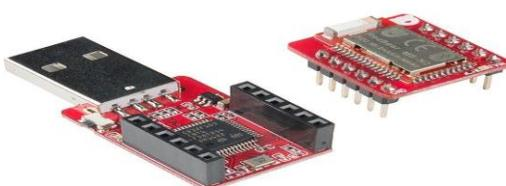
Figure 1. BLE Nano kit microcontroller
